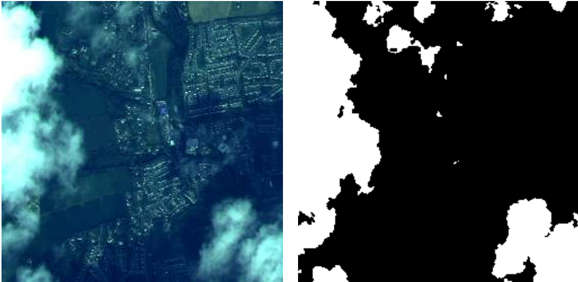
Figure 11: On the left, a scene acquired by WorldView-2. On the right, our cloud map computed according the MKL combination with a = 3 , \log \epsilon = 7 and s = 100 . Notice that the features A and R are ineffective because the pushbroom has only one shift, so that green and blue bands are synchronized. The cloud map is correctly estimated, in particular in the translucent regions located on the top and with few false alarms.
