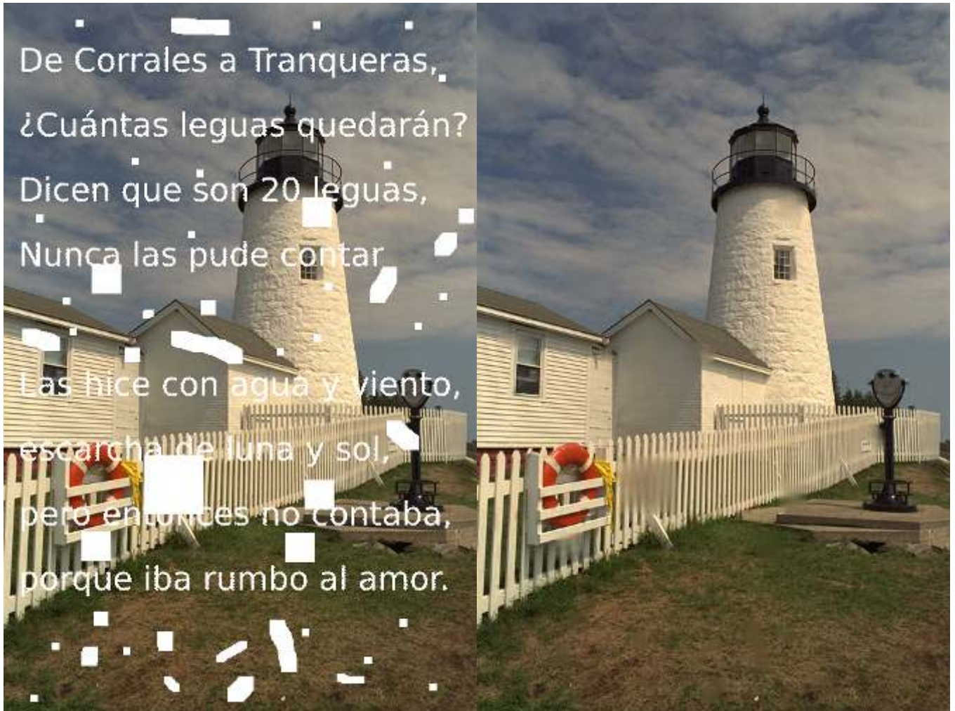
Figure 7: Color image inpainting: sample result for Kodak image #19 and mask #2. Left: overlay of original image and missing pixels mask. Right: Result of applying PACO-DCT with patches of size 64 \times 64 and a stride of 4 pixels (please zoom in on digital document for details). According to Figure 5. Overall, the restored image is visually similar to the original in most regions; the metric SSIM = 0.9678 is consistent with this. On the other hand, the result is not as good on regions which exceed the patch size by a large margin; this explains the relatively high RMSE = 19.85 .
