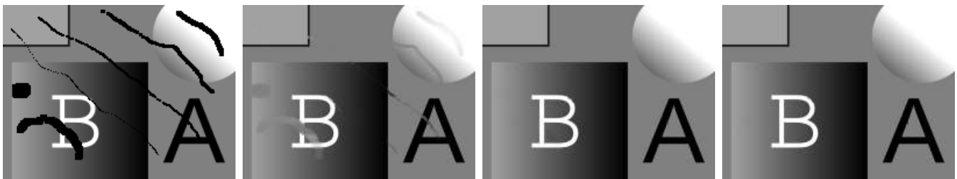
Figure 4: Inpainting results on artificial test image using fully overlapped patches of size 10 \times 10 . Left to right: input image; result after first iteration; result after 16 iterations; after 256 iterations. The first iteration is the result of estimating each patch by minimizing our DCT-based cost function once, followed by a plain patch averaging step, that is, with no consensus imposed.
