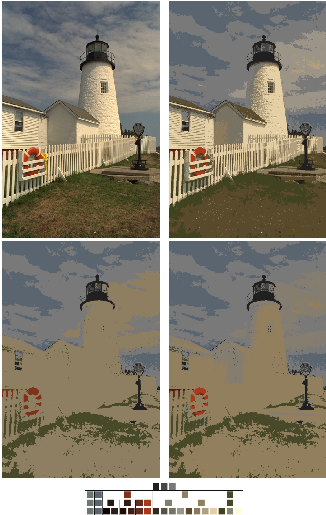
Figure 8: From left to right and from top to bottom: original image, final segmentation, H-segmentation, HS-segmentation and gray+color palette. The gray palette is composed of 3 gray levels and the color palette of 19 colors.
