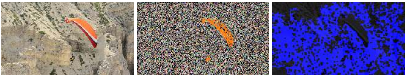
Figure 29: JPEG forgery in an uncompressed image, its vote map and result. An example of wrongly attributed detection: a JPEG compressed image has been pasted into an uncompressed image. The only JPEG traces are the ones in the forged part, which is large enough to result in a global detection. Indeed, this part is larger than 1/64th of the image. The method correctly detects the missing JPEG grids in the background. The result is that the background is marked as forged, while it is more natural to say that the small region is the forged one.
