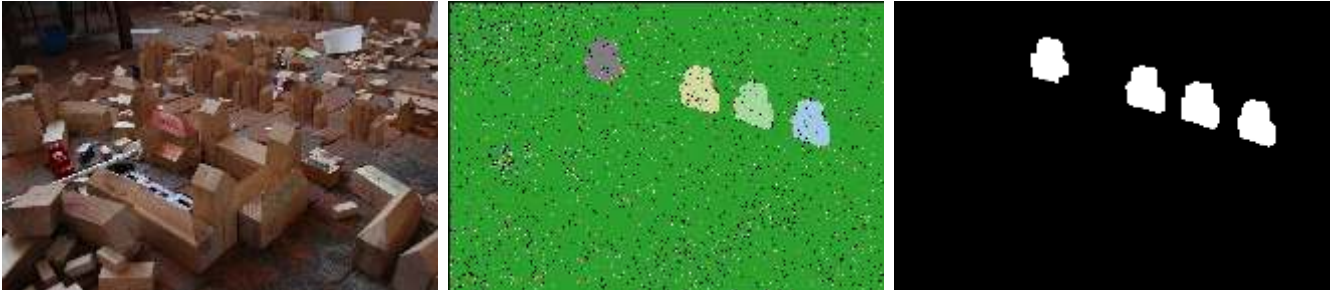
Figure 16: Left: tampered image by copy-move. Middle: vote map. Right: forgery mask F .
