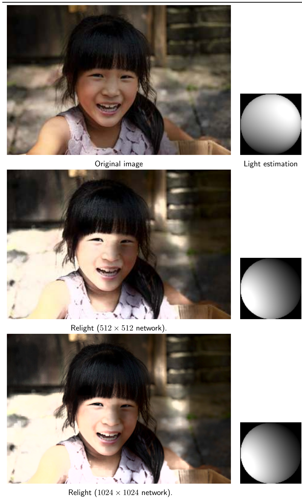
Figure 7: Working on 512 \times 512 images, details are lost and artifacts created when large-scale images need to be resized by bilinear resampling. The 1024 \times 1024 network only partly alleviates this issue. Full resolution versions of the images in the middle and bottom rows can be found in the demo's archive, at https://ipolcore.ipol.im/demo/clientApp/demo.html?id=429&archive=516158 and https://ipolcore.ipol.im/demo/clientApp/demo.html?id=429&archive=516159 , respectively.
