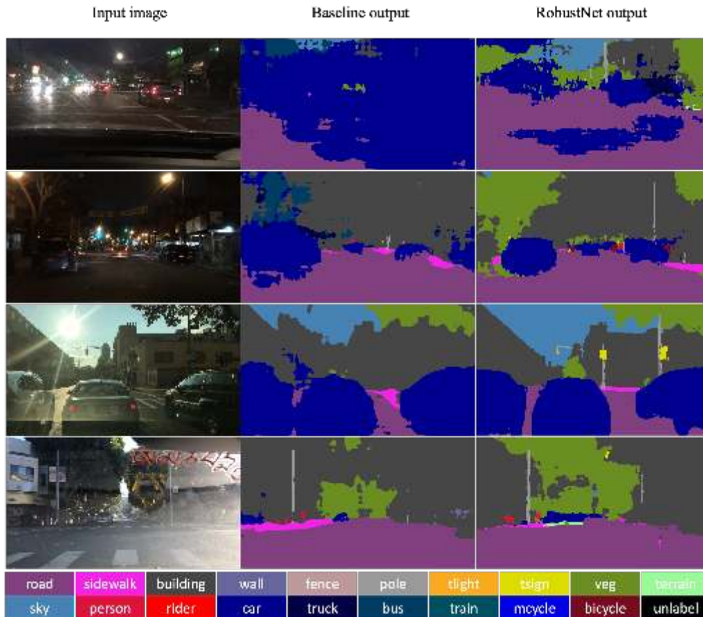
Figure 3: Adverse lightning conditions results for RobustNet. The two upper rows correspond to night , while the two on the bottom correspond to sun reflection . Input images are shown in the left column. In the middle, baseline model outputs are displayed, while RobustNet outputs are shown on the right column. All images were produced with a DeepLabV3+ architecture with ResNet-50 encoder, trained on Cityscapes dataset [4].
