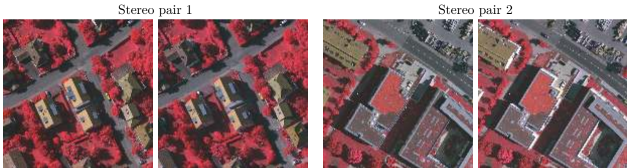
Figure 4: Example stereo pairs from the 2021 aerial stereo benchmark [32], used to fine tune the PSM and HSM networks.
