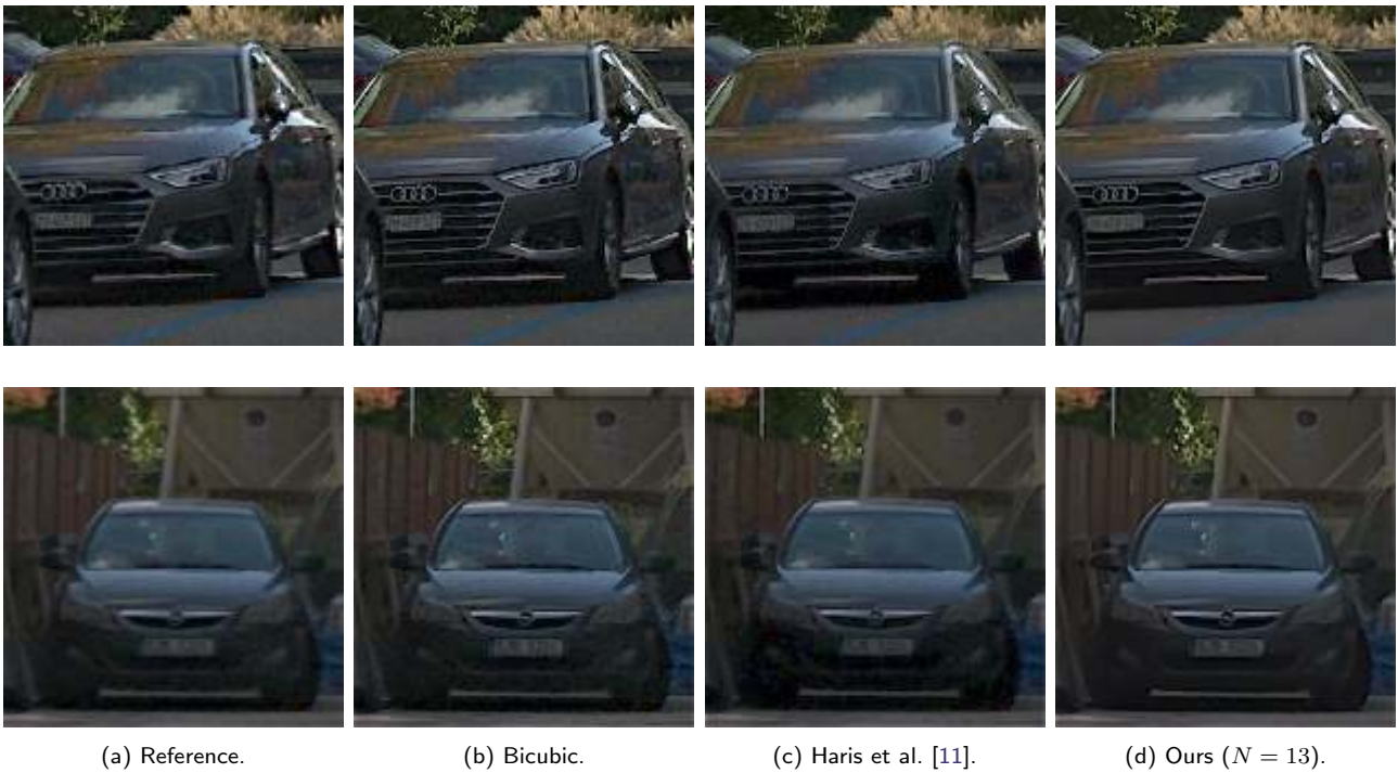
Figure 9: Comparison of different methods for \times 2 zoom on a real burst from [3]. The images are demosaicked using [10], upscaled using several methods, then postprocessed using [8]. Our pipeline manages to recover sharp details such as registration plates, while denoising even the darkest areas. Better seen by zooming on a computer screen.
