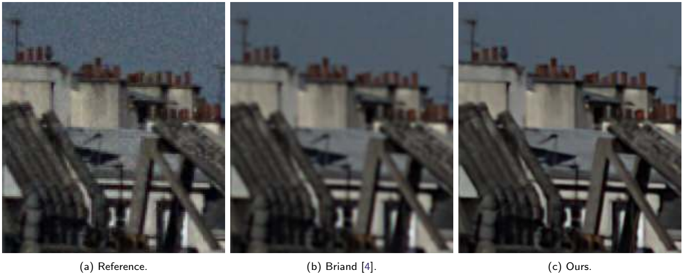
Figure 13: Comparison of locally adaptive anisotropic kernel and the general isotropic kernel from [4] for \times 2 zoom from a burst of N = 20 raw images. Our kernel is narrower than the isotropic counterpart for punctual details like the chimneys, allowing for sharper details. For texture-free areas like the sky, our kernel gets wider than that of [4], allowing for a more efficient denoising. By stretching on edges, our kernel is less prone to create blue and red stripes artifacts on edges. The images are not sharpened for better highlighting the disparity of the remaining blur straight after image fusion.
