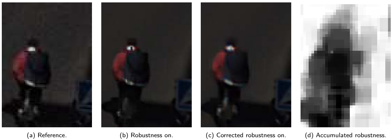
Figure 12: Illustration of the additional frame-count aware spatial denoising for a \times 2 zoom of a real 20 images burst. With the mere robustness logic, patches with a low accumulated robustness (black pixels in Figure 12d) are mostly obtained using single-frame SR and are therefore exceptionally prone to demosaicking artifacts and noise (Figure 12b). By adapting the merge kernel of the reference frame to the accumulated robustness (Figure 12c), fine details such as the bicycle frame remain visible and merge artifacts disappear. Note that for illustration purposes the images are not post-processed using [8], which would completely remove the color flutter of the artifacts.
