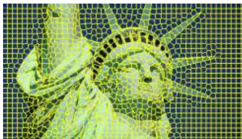
Figure 1: Visualization of a superpixel segmentation S obtained with the SLIC algorithm [1, 5].
