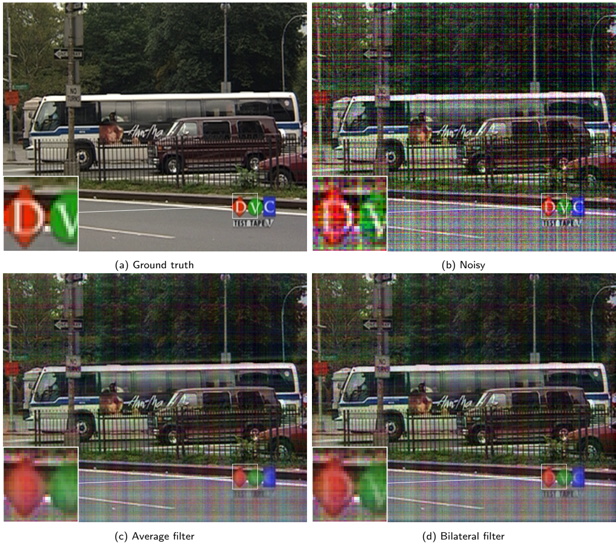
Figure 6: Comparison of the different methods on the last image of the bus dataset that contains 150 frames and some motion. Simulated additive and multiplicative FPN, spatially structured and spatially independent, with a standard deviation of \sigma_{bw} = \sigma_{br} = 15 , \sigma_{aw} = \sigma_{ar} = 0.10 was added to the frames. (a), (b), (c), (d) are respectively the ground truth clean image, the noisy image with simulated FPN, the image denoised by an average filter and the image denoised by a bilateral filter.
