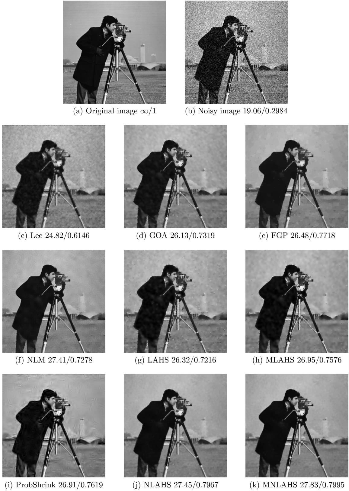
Figure 7: The results of the proposed method in comparison with several noise suppression methods. (a) Original image, (b) Noisy image ( \sigma_n = 30 ), (c) Lee, (d) GOA, (e) FGP, (f) NLM, (g) LAHS, (h) MLAHS, (i) ProbShrink, (j) NLAHS, and (k) MNLAHS. The PSNR/SSIM values are shown below the images.
